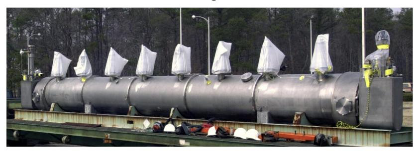
Usually 8 Cavities per Cryomodule
