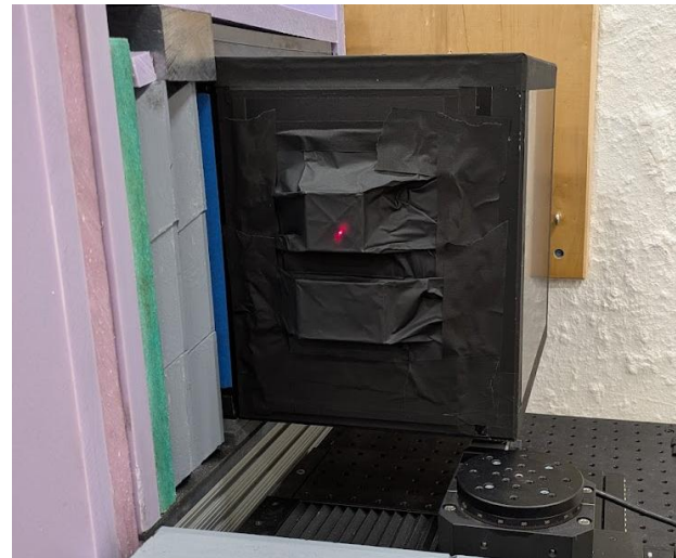
CapeSym Detectors in Fast Neutron Beam
