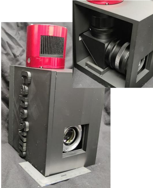
Compact Camera Prototype Smaller Field of view, Higher Magnification
