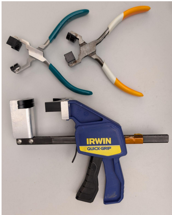
Tooling to bend ends
