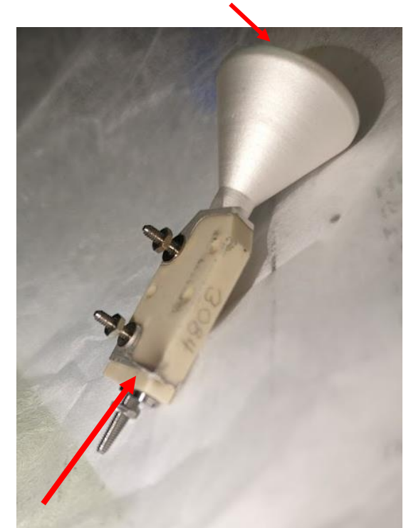
Contact from redesigned metallization caused shorts
