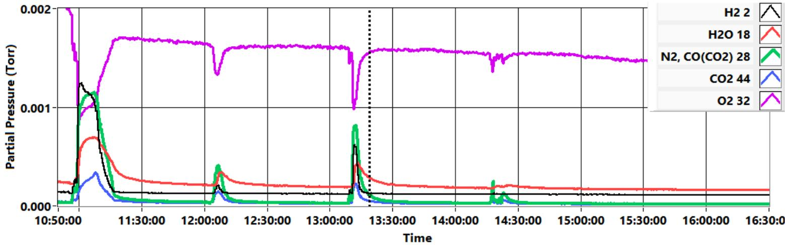
• The violet trace which is oxygen, the lower plot are the hydrocarbon residuals of hydrogen, water, carbon monoxide and carbon dioxide.
