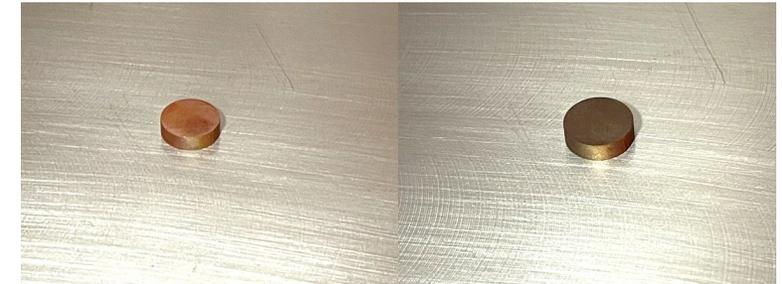
excessive oxidation due to heating during plasma processing
