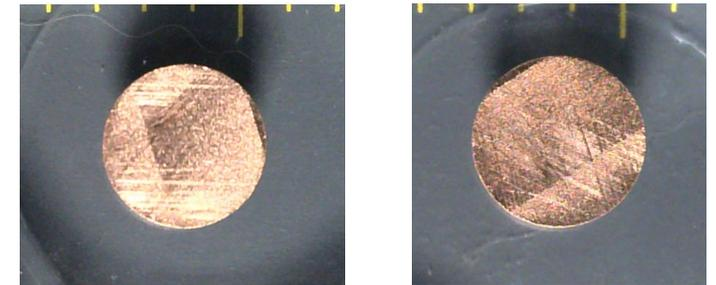
No excessive oxidation observed at reduced power and shortened cycles in plasma processor
