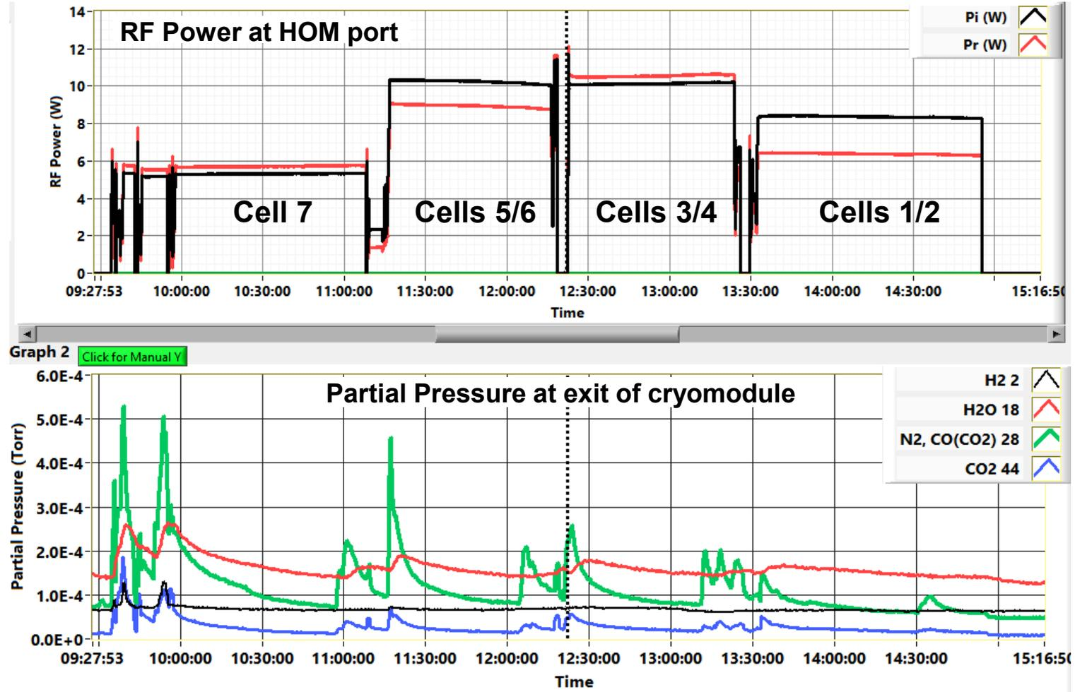
Extra peaks in the hydrocarbon residue plots occurred when we moved the plasma from cell to cell in other cavities in the cryomodule.
