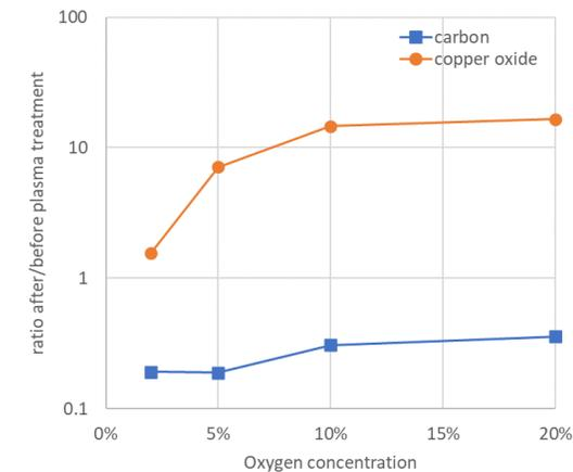
Higher oxygen concentration leads to largest increase of work function but also increased oxide layer
