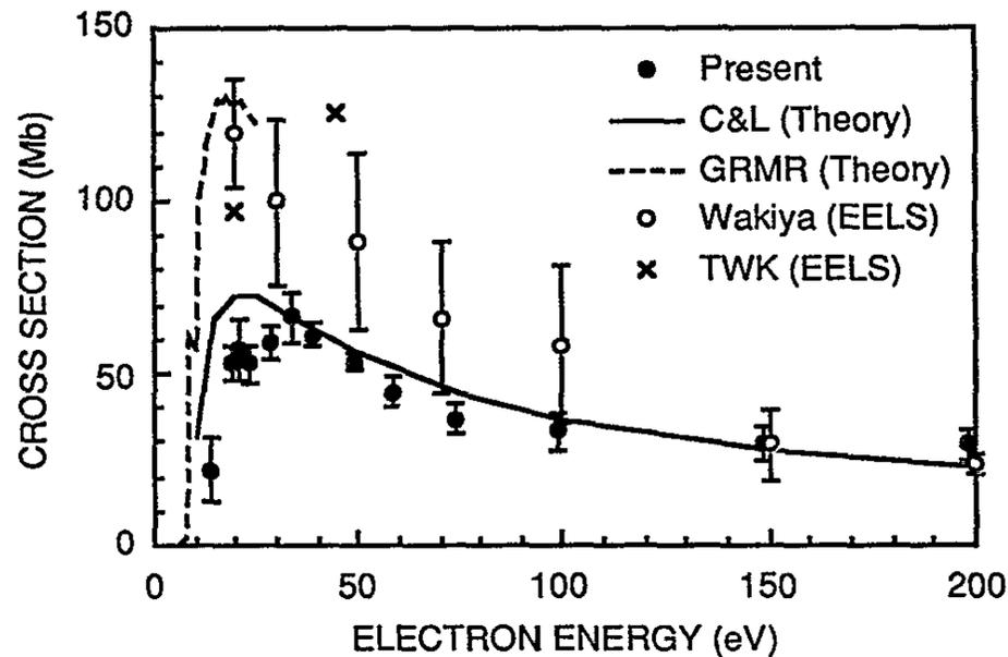
Dissociation Cross Sections and excitation cross sections for electron impact on O<sub>2</sub>\*\*
