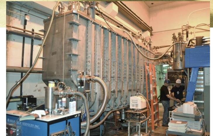
2019 ANL/FNAL half-wave cryomodule for PIP-II
