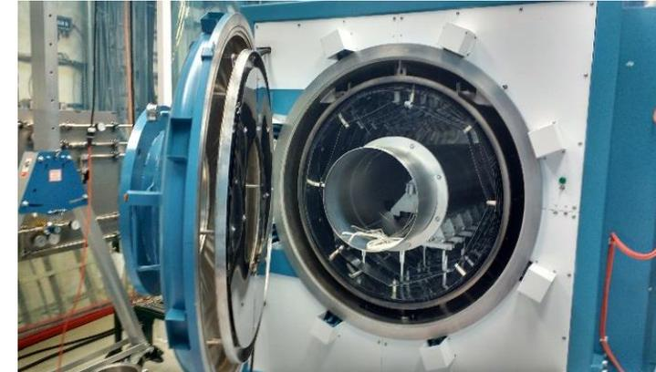
Nb<sub>3</sub>Sn coating furnace at Fermilab
