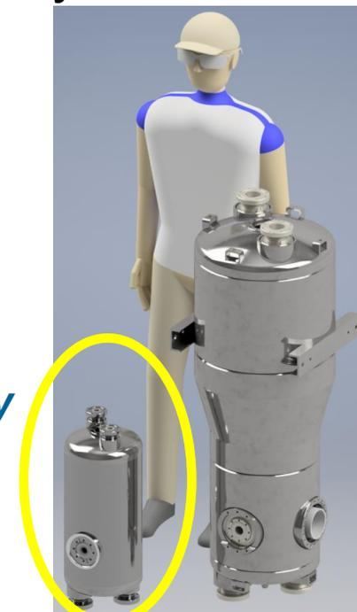
New 218 MHz QWR and existing ATLAS 72 MHz cavity
