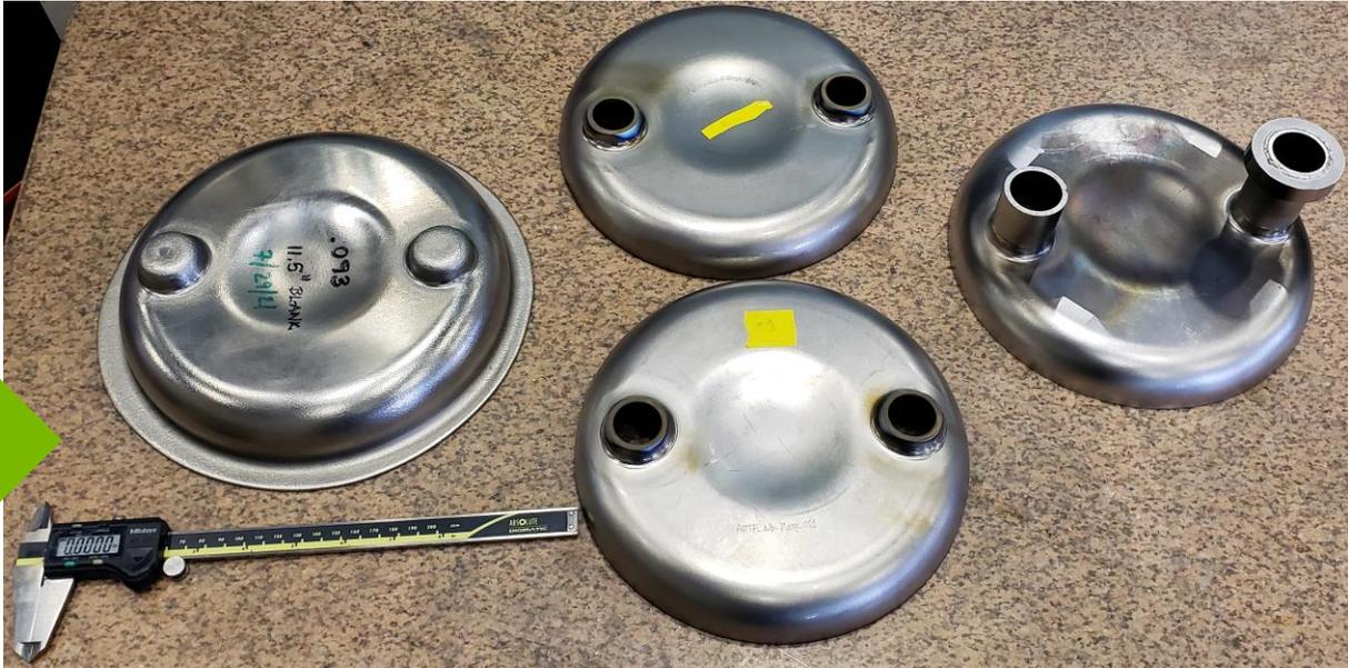
'low RRR' test (left), production parts (middle), test dome w/ ports (right)
