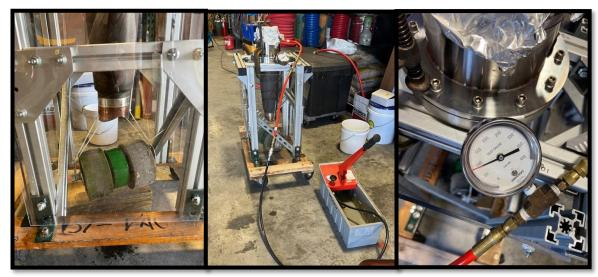
The test assemblage with the added weight, the manual water pump connected to the setup ready for the hydrostatic pressure test, and pressure gauge showing 98 PSIG of water pressure
