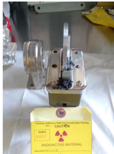
damaged beamline valve damaged magnet and cables
