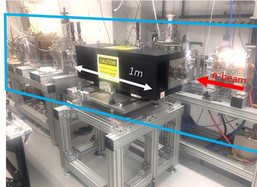
Section of AWA beamline used in the experiment. Wiggler was assembled using spare magnetic structures and a new strong back frame and a new vacuum chamber. Wiggler period = 8.5 cm, K=10.8
