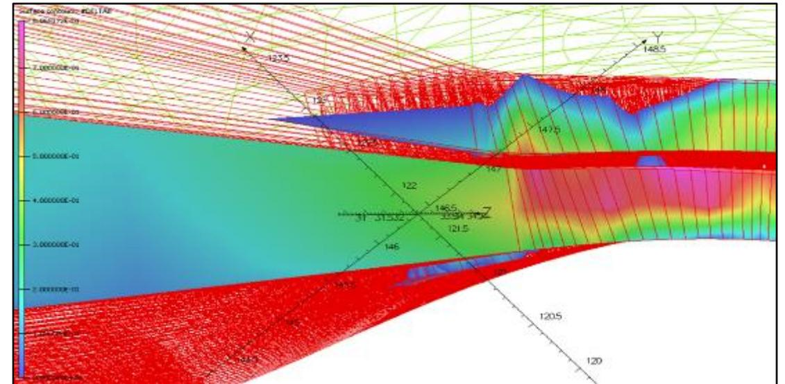
**Fig. 2: Peak field in the magnet ends vs. straight section with the modified geometry [5].**
