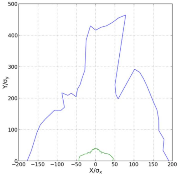
Dynamic aperture for the bare lattice (blue) and with one b6 systematic multipole in the first upstream FFQ (green) [8]
