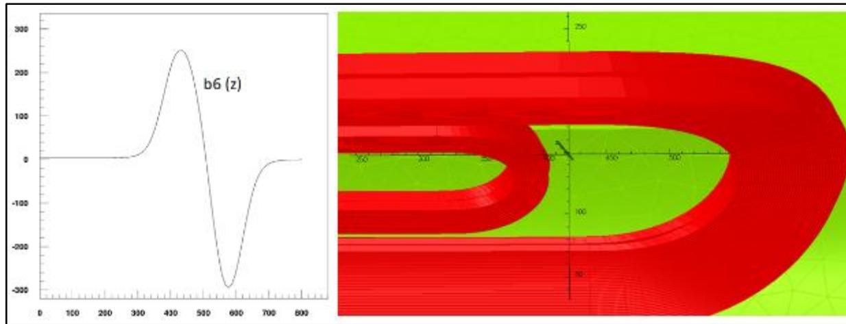
**Fig. 1: Modified end configuration for canceling the  $b_6$  integral [5].**
