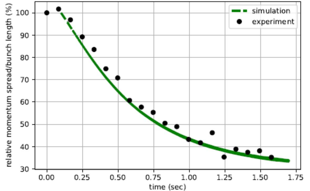
Cooling of krypton ion bunch with 500 ns electron bunch
