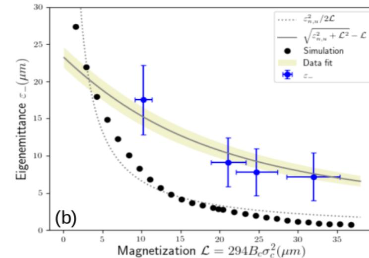
Eigen emittances of the 3.2 nC magnetized beam experimentally measured at FAST (blue circles with error bars) compared with numerical simulations carried out with IMPACT-T.
