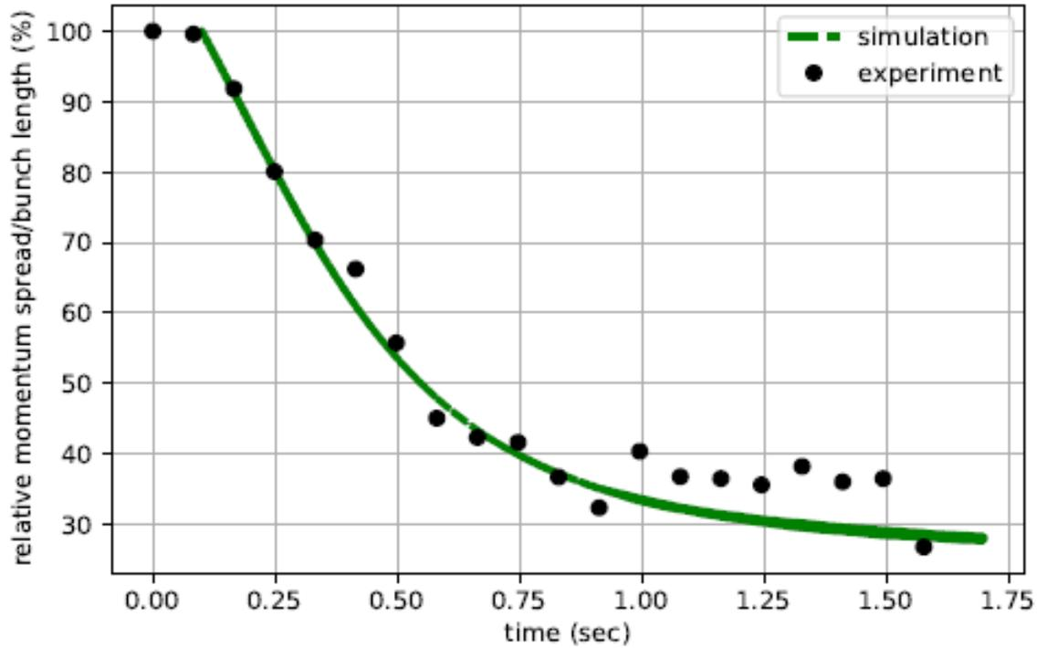
Cooling of krypton ion bunch with 900 ns electron bunch
