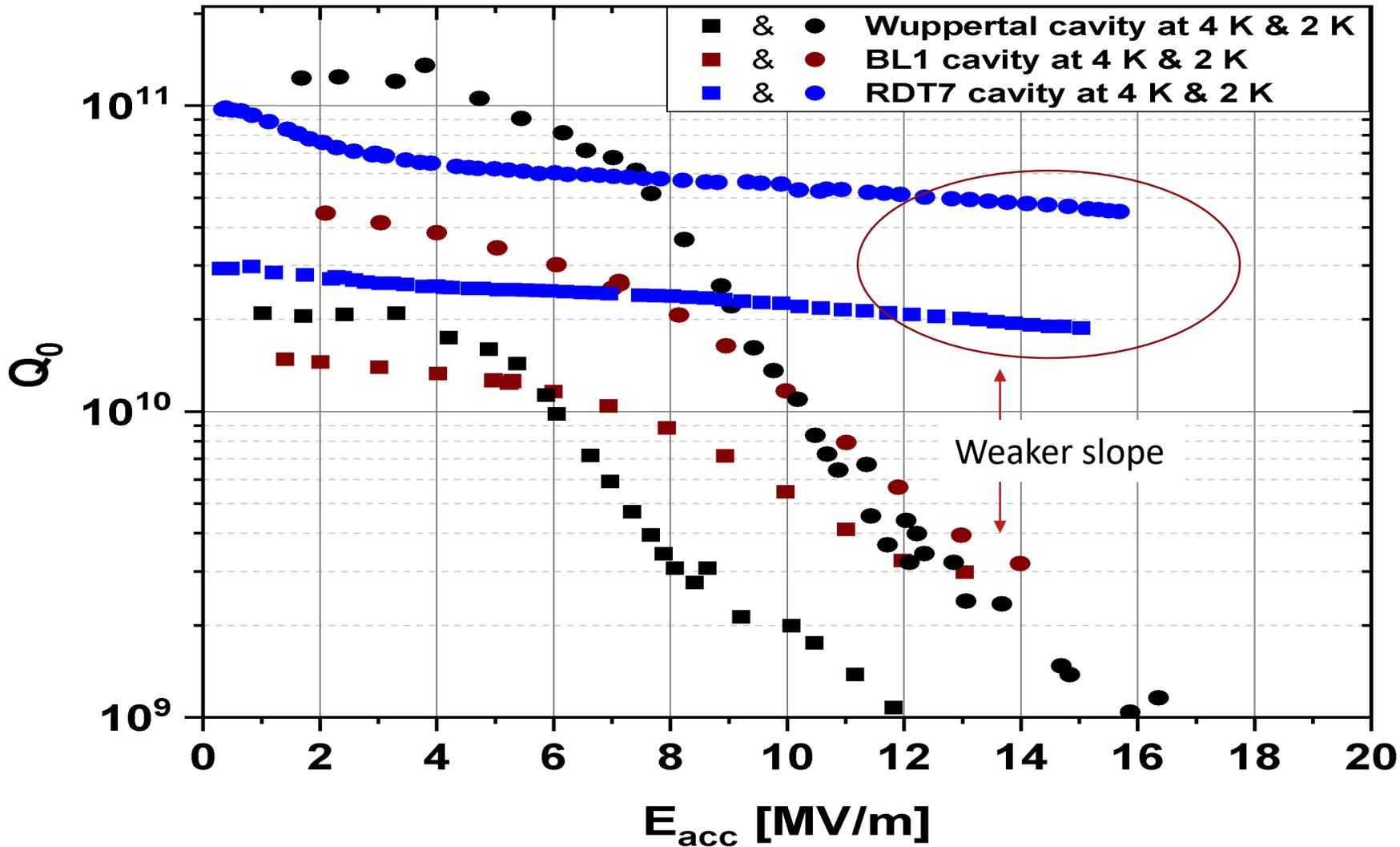
Following titanium hypothesis, during the coating system upgrade efforts were made to avoid any potential titanium sources. Only all niobium cavities are allowed to be coated now. NbTi flanges were replaced with Nb flanges on RDT7.
