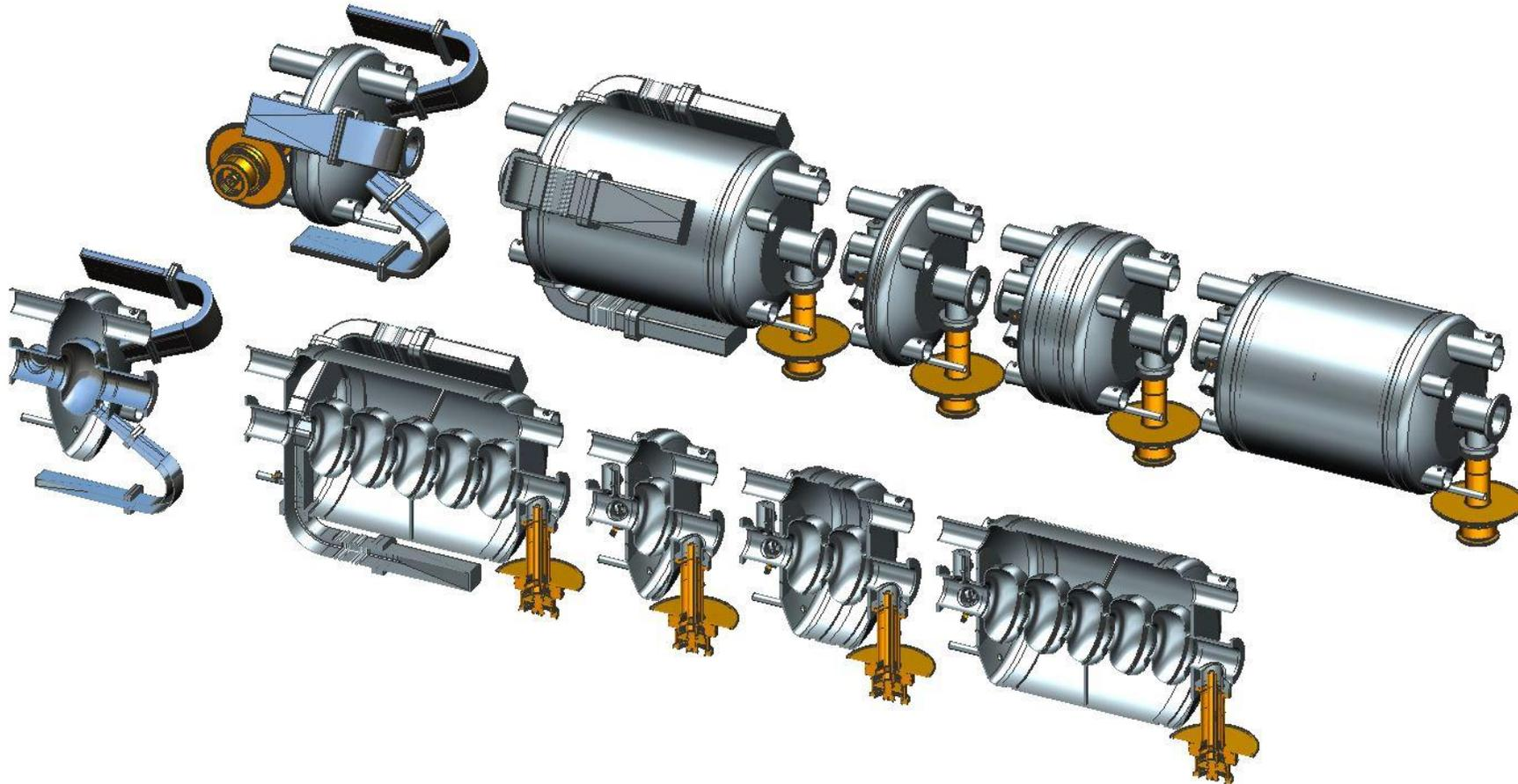
1 to 5 cells, coax, WG or on-cell dampers
