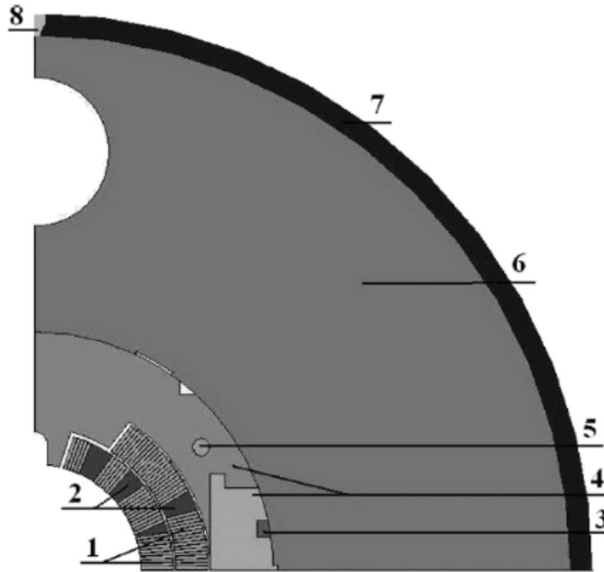
Fig. 1. Cross-section of the dipole (one quadrant is shown). 1-coil, 2-inter-turn spacers (wedges), 3-key, 4-collars, 5-pin, 6-yoke, 7-outer cylinder, 8-weld.
