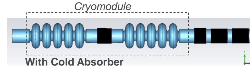
**Conclusion: HOM damping with only beamline absorbers can provide strong damping; a cold absorber is necessary to avoid potential trapped modes**
