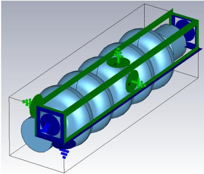
Beampipe with SiC Rings: Transmission Line
