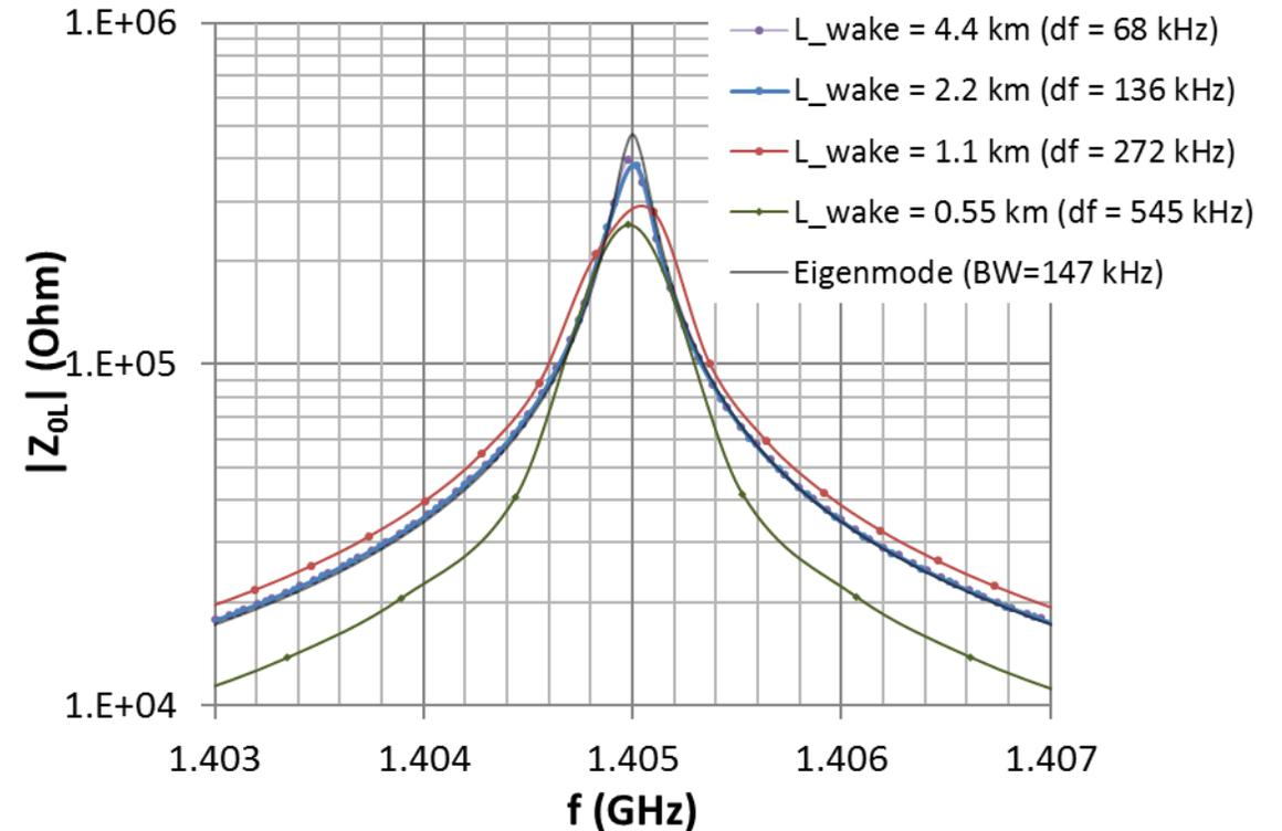
**Conclusion: Peak impedance and apparent Quality factor (damping) are a strong function of the wake integration time and the mesh**
