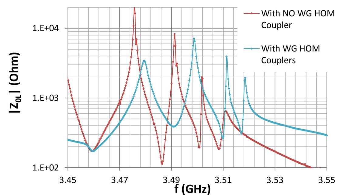
**Conclusion: The ridged waveguide assembly alone is insufficient; some monopole modes only strongly coupled to the beam tube, i.e. the location of a beamline HOM damper**
