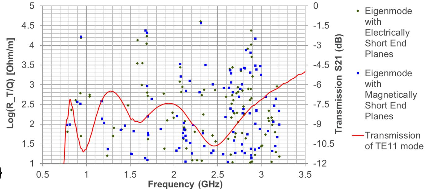
**Conclusion: Possible to optimize dimensions of the silicon carbide rings for strong damping at highest  $R_T/Q$ ; We take advantage of intrinsic property of the SiC ring as a broadband dielectric resonator**
