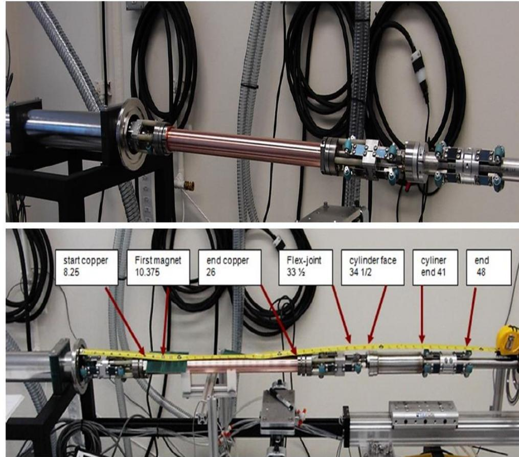
Figure 6.206: Magnetron coating mole: Top: 50 cm long cathode magnetron. Bottom: the 50 cm long cathode magnetron assembly; the magnetron carriage has spring loaded guide wheels that cross bellows and adjust for diameter variations keeping the magnetron centered.
