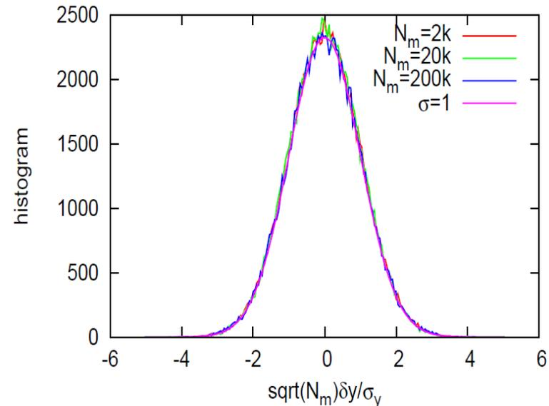
The plot on the right shows that between 2k and 200k particles the RMS fluctuation in the electron centroid is just statistical.
