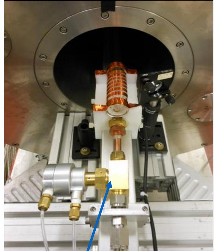
**Non-magnetic brass pneumatic remotely controlled Isolation Valve**
