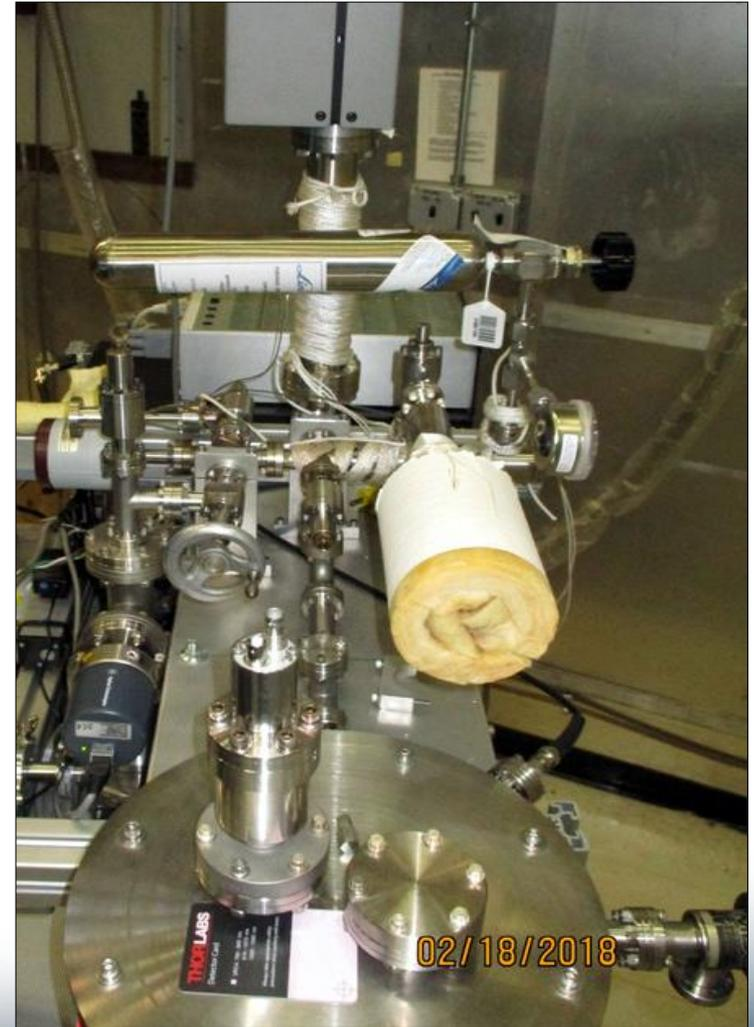
**$^3\text{He}$  cryo- purification system built-in CTI-8 cryo-pump.
