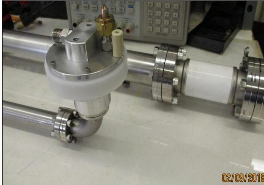
*In the 2.0 T solenoid field the 1.0" long insulator is holding 40 kV voltage difference in between valve and drift tube up to 0.1 Torr He-gas pressure "magnetic isolation".*
