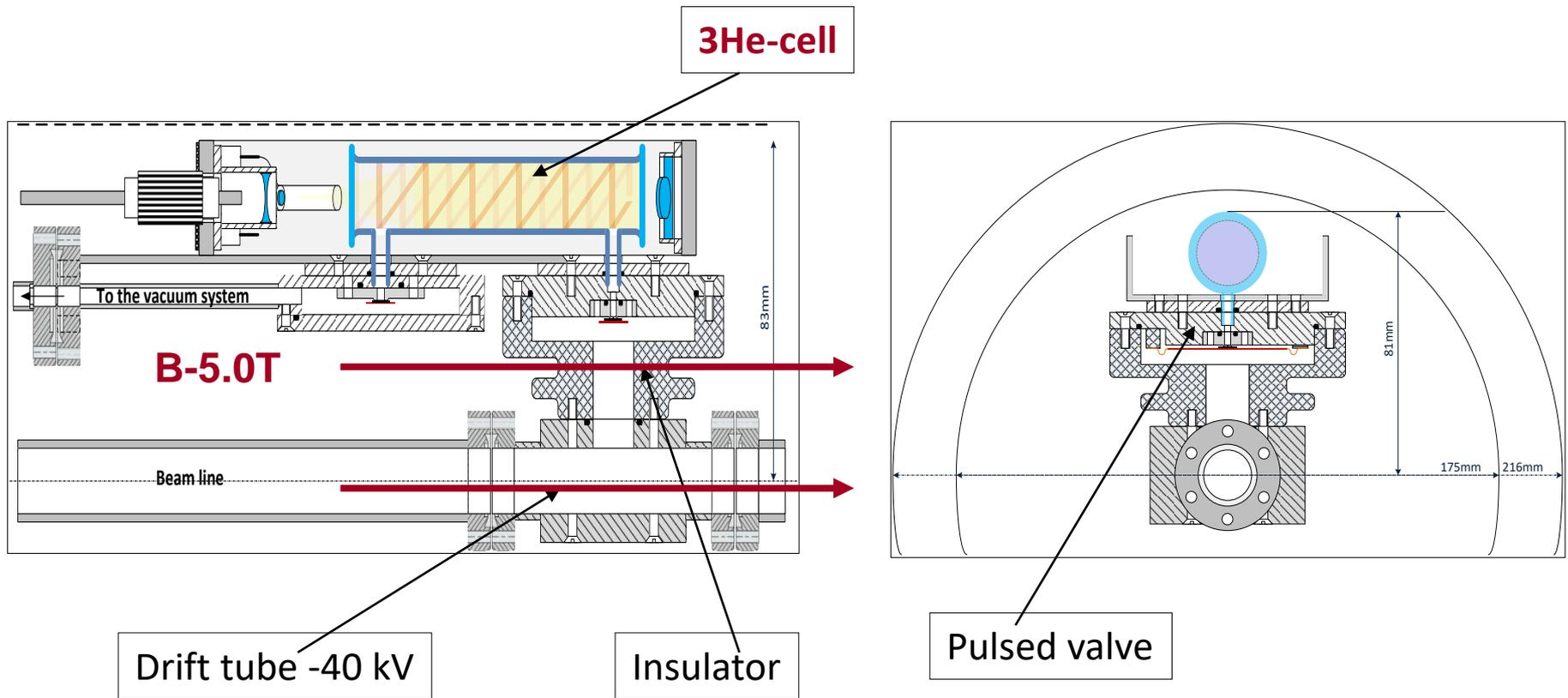
Long, small diameter drift tube works like a  $^3\text{He}$  storage cell, which reduces gas load to the EBIS vacuum system and increases polarization due to ionization localization in the high magnetic field region.
