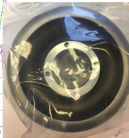
First known use of stainless steel 3D printing for a XHV part. Outgassing study indicate superior performance compared to conventionally construction.
