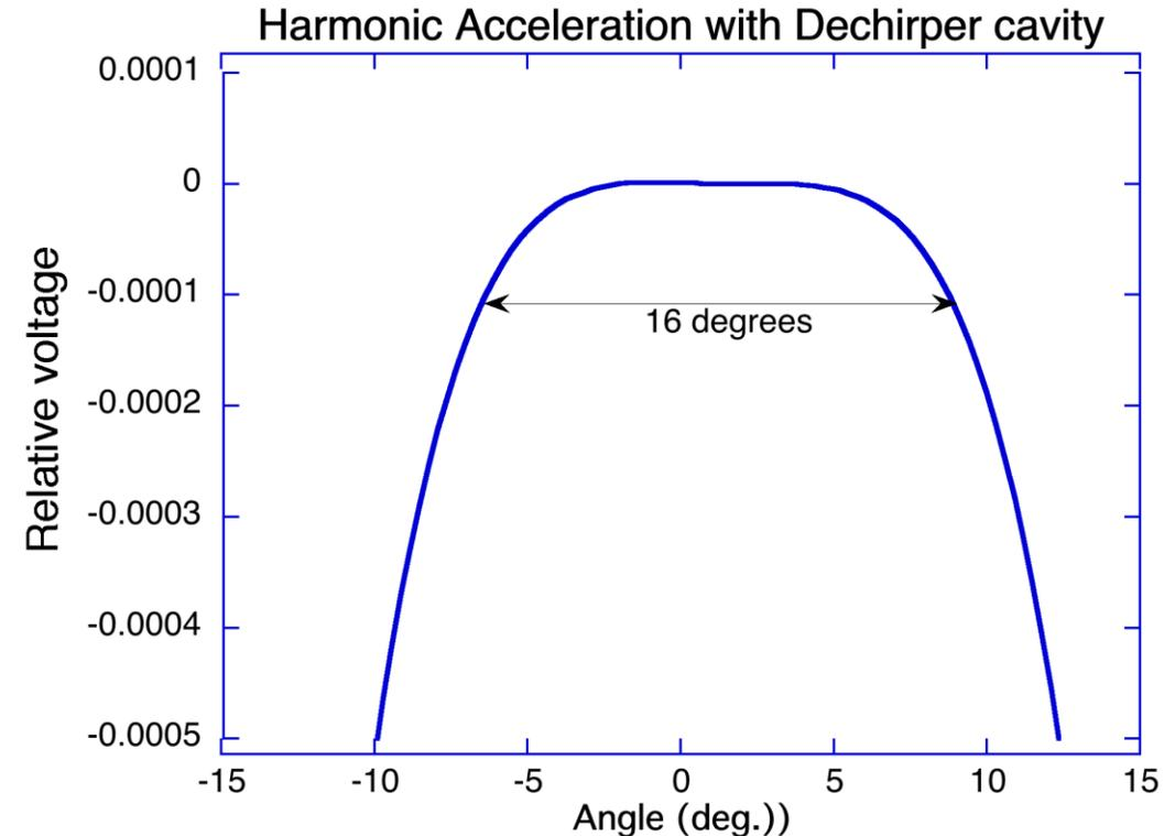
Before going into the CCR, take out the slope using a 952.6 MHz de-chirper.
