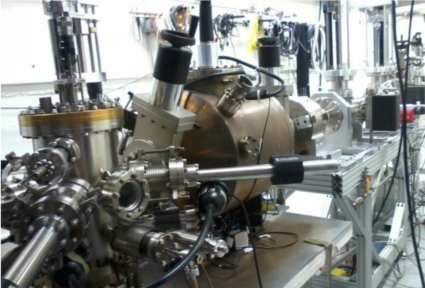
**Always something to fix:** Valve between gun and depo chamber leaked, working distance between puck and chemical sources too large, no mask to limit active area
