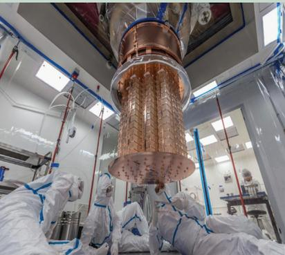
Figure 4: The CUORE experiment used radon-free environments to assemble and install the bolometer towers. | Image reproduced with permission from Yury Suvorov, University of California Los Angeles and Gran Sasso National Laboratory (Italy), and the CUORE Collaboration.
