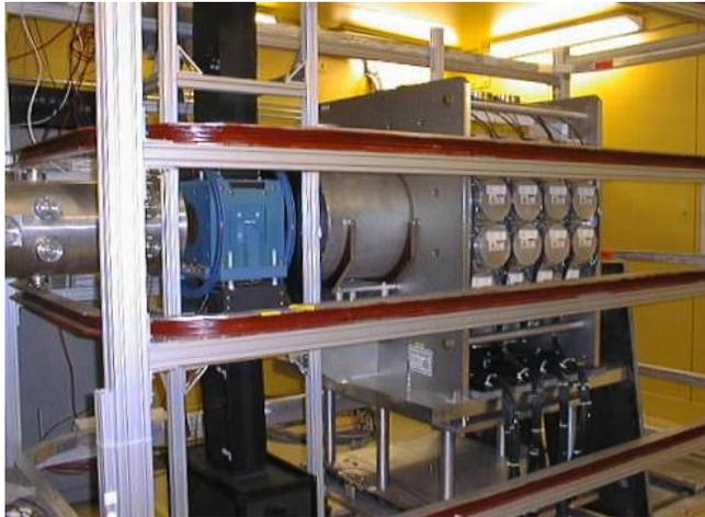
*Polarizer, Field Coils, Spin Flipper, & Detector*
