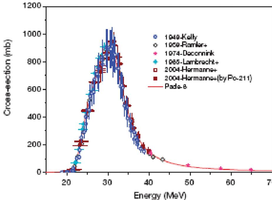
FIG. 2.4.2. Excitation function for the  $^{209}\text{Bi}(\alpha, 2n)^{211}\text{At}$  reaction.
