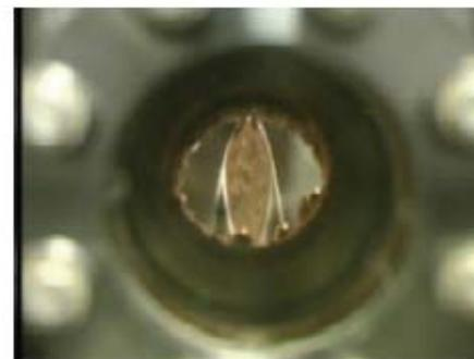
A thin film of liquid lithium  $\sim 420 \mu\text{g}/\text{cm}^2$  thick moves at  $\sim 70$  meters per second from the top to the bottom of the opening. A beam of Uranium ions will be passed through the film to strip away atomic electrons so that the uranium ions can be accelerated to the full energy of the FRIB.
