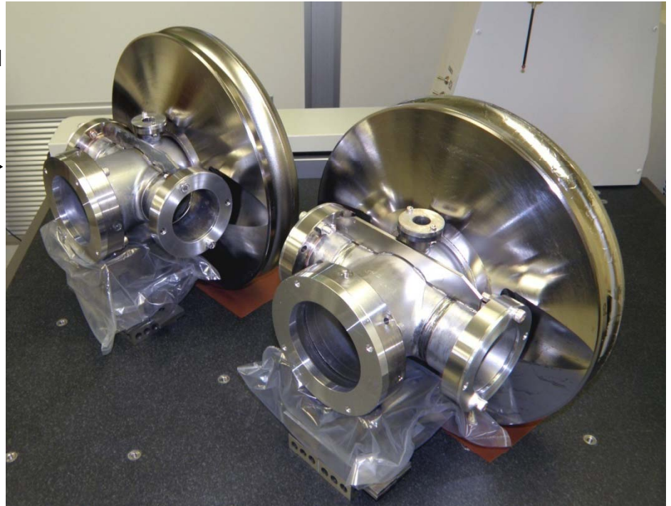
Superconducting electron gun, developed at BNL by DOE in cooperation with DOD and industry.
