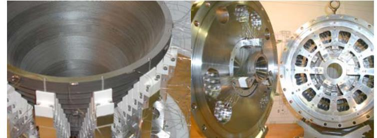
Gas catcher technology developed, tested and now routinely used at ATLAS for CPT and RIA programs
