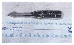
Figure 9: Determination of the characteristics of an unknown interdicted sample often relies on isotopic measurements and certified isotope reference materials. The glass ampule shown (interdicted in Bulgaria) was determined to contain highly enriched <sup>235</sup>U
