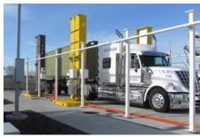
Figure 5: Portal monitor containing <sup>3</sup>He in use scanning a cargo containing truck
