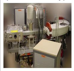
Figure 12: INL stable mass separator
