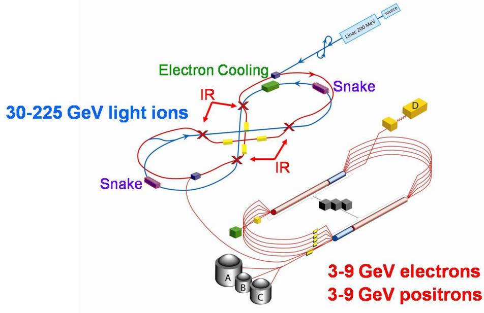
Figure 28: Design layouts of the ERL-based eRHIC, and the CEBAF-based ELIC colliders.
