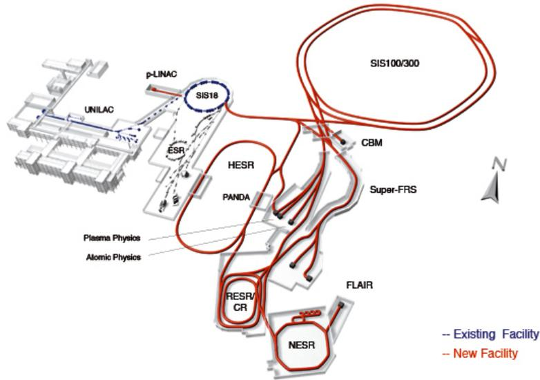
Figure 29: The Facility for Antiproton and Ion Research at GSI showing the exiting components and the planned new construction. The focus for hadron physics will be on research with precision, cooled, stored beams of antiprotons.
