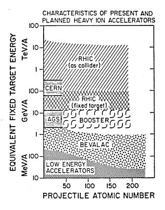
The role of a medium-energy heavy-ion accelerator can be placed in the context of a structured national program of heavy-ion research. Different accelerators in different energy regimes address a range of different nuclear physics questions as was the case in the structured program of electromagnetic research. As Figure 3 shows, the very highest energies for
