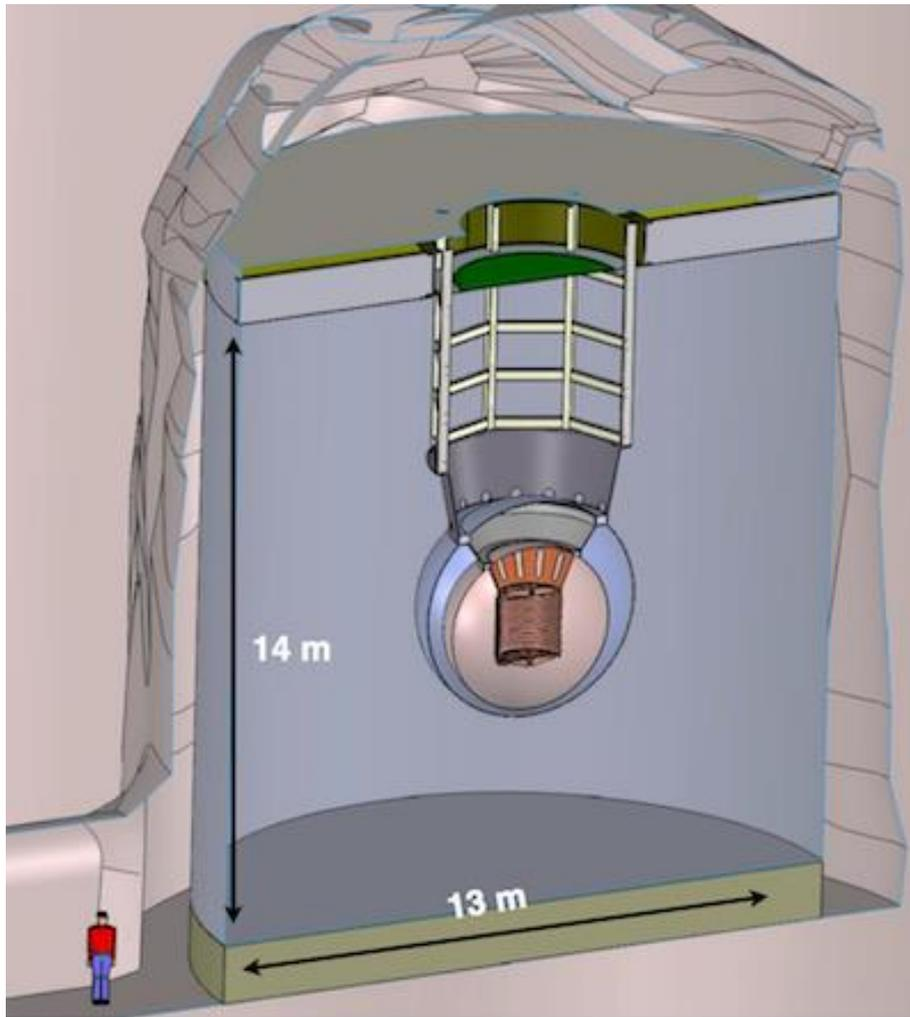
Artist rendering of the nEXO TPC (left) and its installation at the SNOLAB cryopit (left). The cryostat is submerged in a water tank which acts as active shielding. SiPMs will be mounted between field shaping rings and detector wall.
