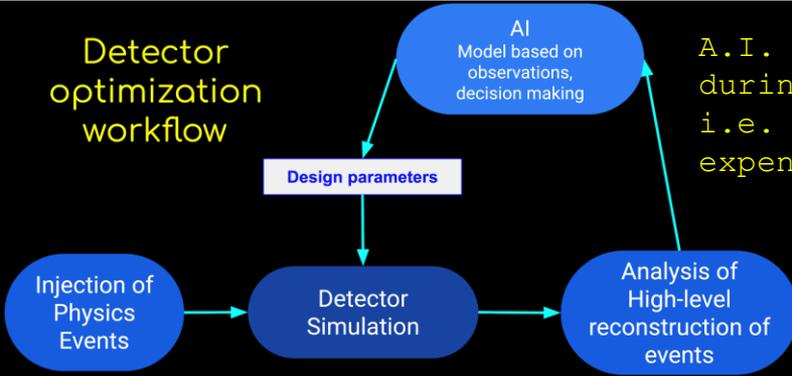
A.I. can optimize the design of complex during the R&D of large-scale detectors, i.e. simulating noisy and computationally expensive black-box functions
