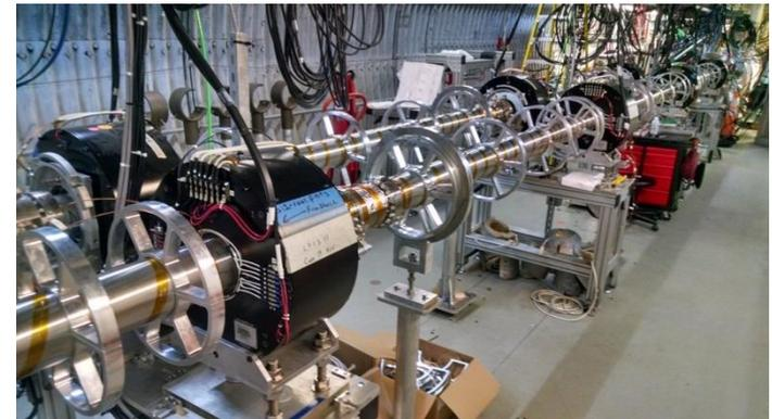
Cooling of low energy, bunched heavy ion beams (3.85–5.75 GeV/n) to increase luminosity
