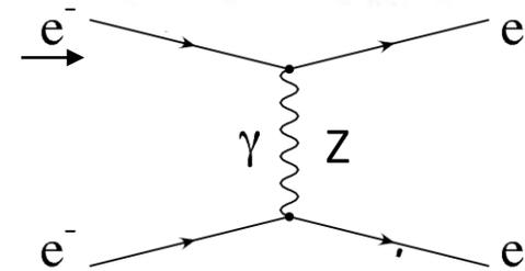
In MOLLER, polarized electrons are scattered off unpolarized electrons. The amount of parity violation due to interference of the two possible exchange mechanisms ( $\gamma$  or  $Z$ ) is precisely predictable in QED. (No messy quarks or color charge, or QCD to worry about, only quantum electrodynamics). The theory is so “clean” that like the  $g-2$  approach, if the level of parity violation is greater than expected, a new particle must be the source of the discrepancy.
