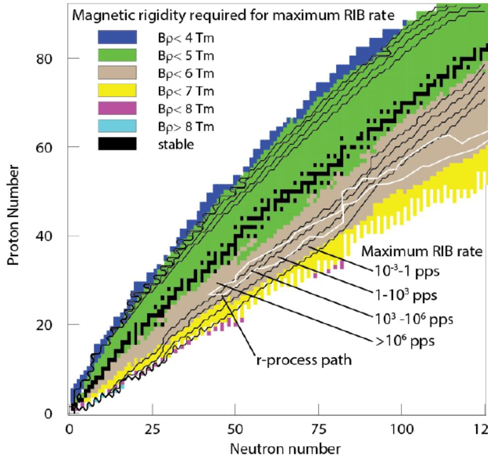
By design, the day-1 physics program will make use of existing NSCL infrastructure. The S800 and Sweeper Spectrometers currently available at NSCL have magnetic rigidity (bending power) limits of 4 Tesla-Meters
