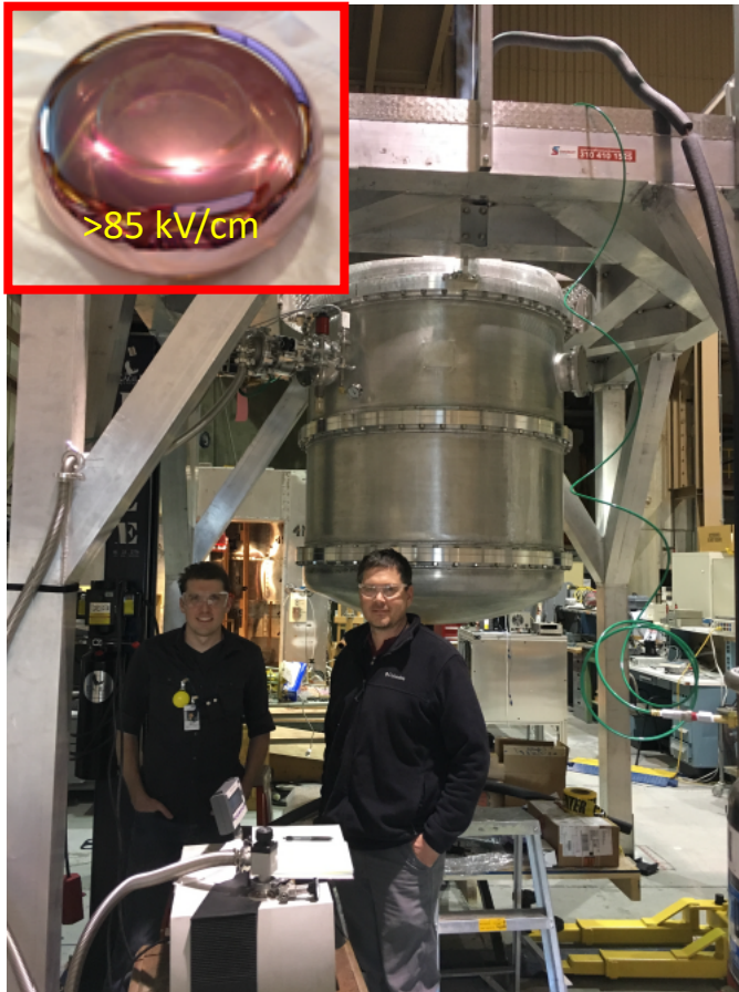
High-voltage Test Cryostat
