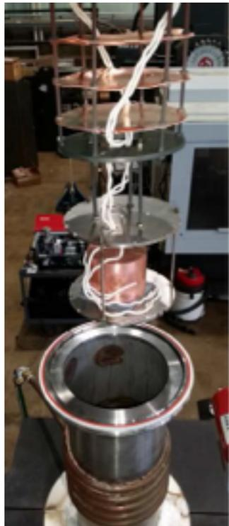
non-magnetic dilution refrigerator under construction
