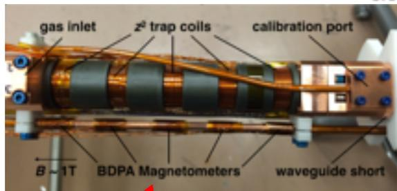
Project 8 Phase II Waveguide Prototype
