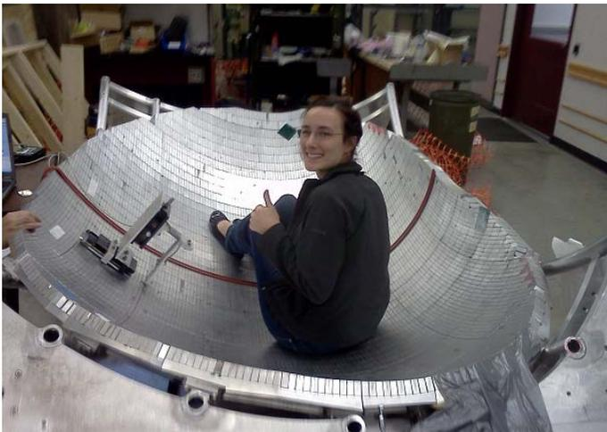
Cubic meter trap stores tens of thousands of neutrons per fill, allowing rapid study of small effects.
