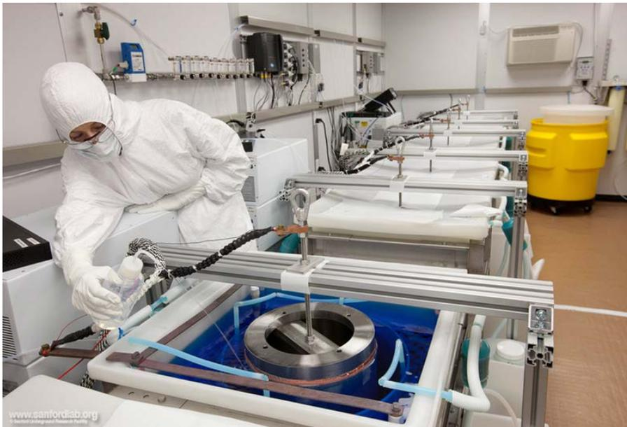
Mandrel insertion in MJD electroforming lab
