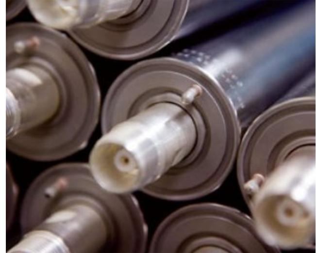
He-3 detector tubes used in Truck Portal monitors
