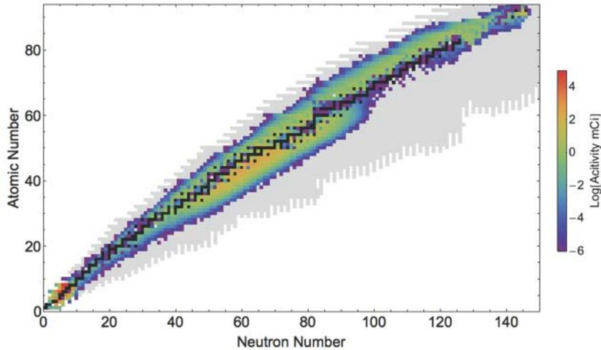
activity produced per day by a 200kW uranium beam stopping in the water beam dump – lots of new and unusual possibilities
