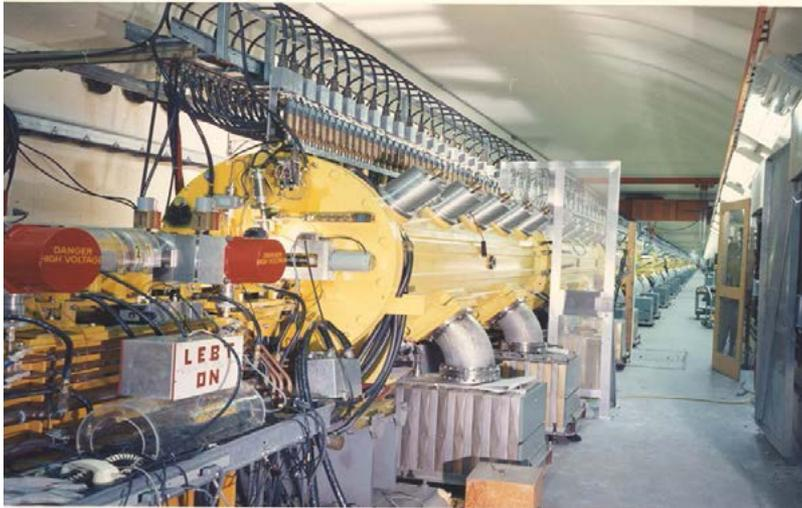
The LINAC supplies protons to the Booster for nuclear physics. Excess pulses (~88-92%) are diverted to BLIP. Energy is incrementally variable from 66-202 MeV.
