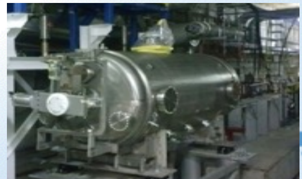
56 MHz quarter wave SRF cavity
