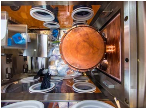
Copper cryostat, as seen from above, will hold the extremely sensitive detector strings. This is a prototype of the ultra-pure copper that will be used in the actual module of the Majorana Demonstrator.
