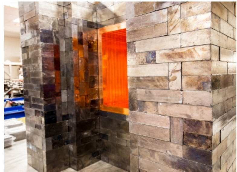
Engineering Majorana's shield: The lead brick "castle" contains 3400 bricks
