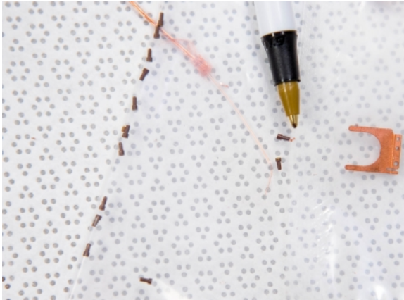
MJD requires precision machining. These tiny parts are made in Majorana's machine shop. These small pins will hold the conductive wire in the copper clip at right.
