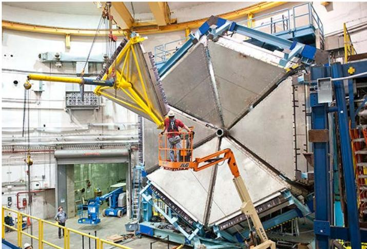
Mounting of the Forward Time-of-Flight detector arrays onto the forward carriage in Hall B
