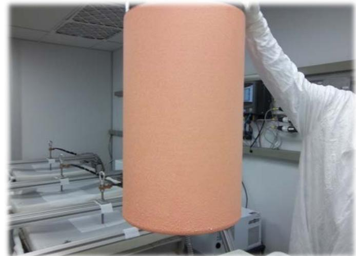
Inspection of copper being electroformed at the Temporary Clean Room in SURF
