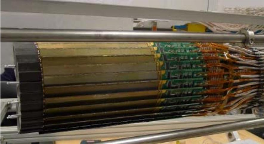
The recently completed STAR Heavy Flavor Tracker to enable measurement of heavy quarks
