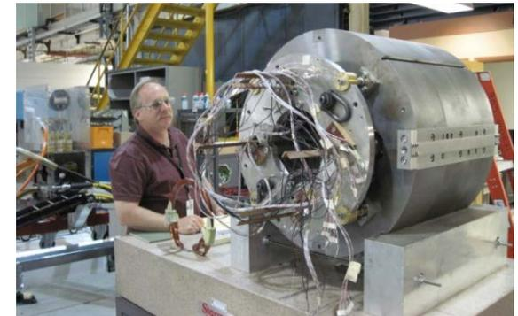
The coils of this high temperature superconducting (HTS) quadrupole exceeded the required currents at elevated temperatures, indicating additional operating current margin and more stability.
