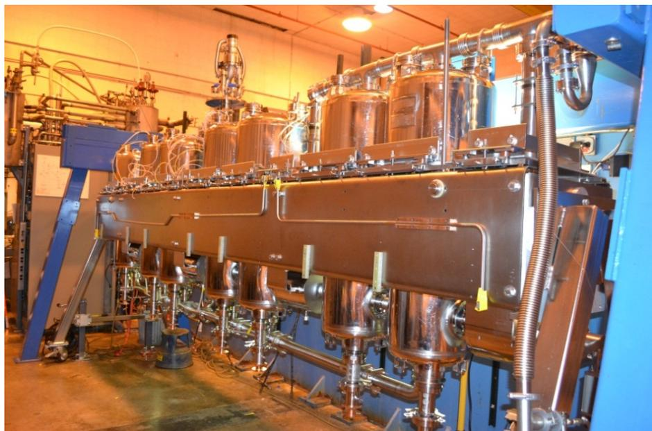
Cryomodule components at ATLAS (ANL)
