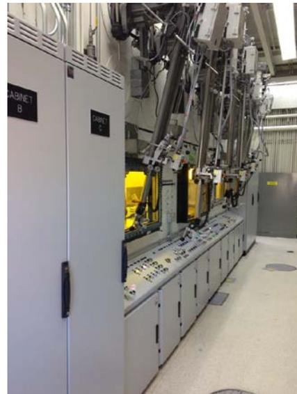
Hot cells used to purify highly radioactive materials for medical use
