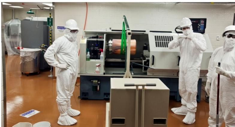
4800 feet below ground, the copper needed for a cryostat to cool sensitive Germanium detectors is being electroformed to avoid induced backgrounds caused by cosmic rays
