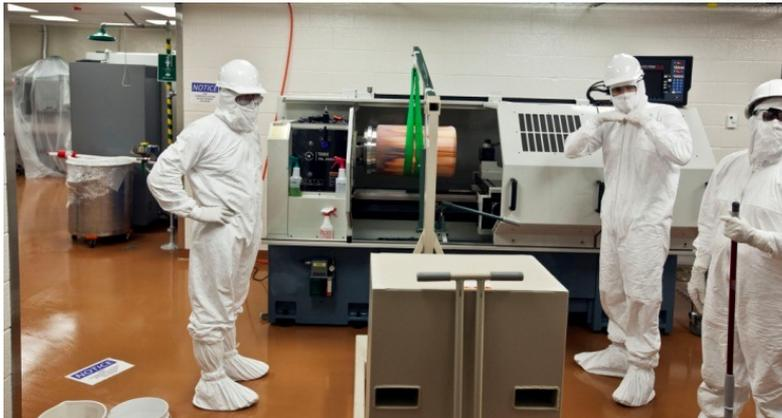
4800 feet below ground, the copper needed for a cryostat to cool sensitive Germanium detectors is being electroformed to avoid induced backgrounds caused by cosmic rays
