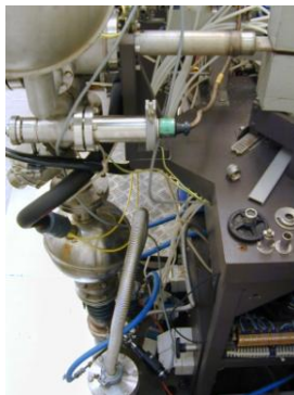
mercury pump for ion source (replaced by ion getter pump)
