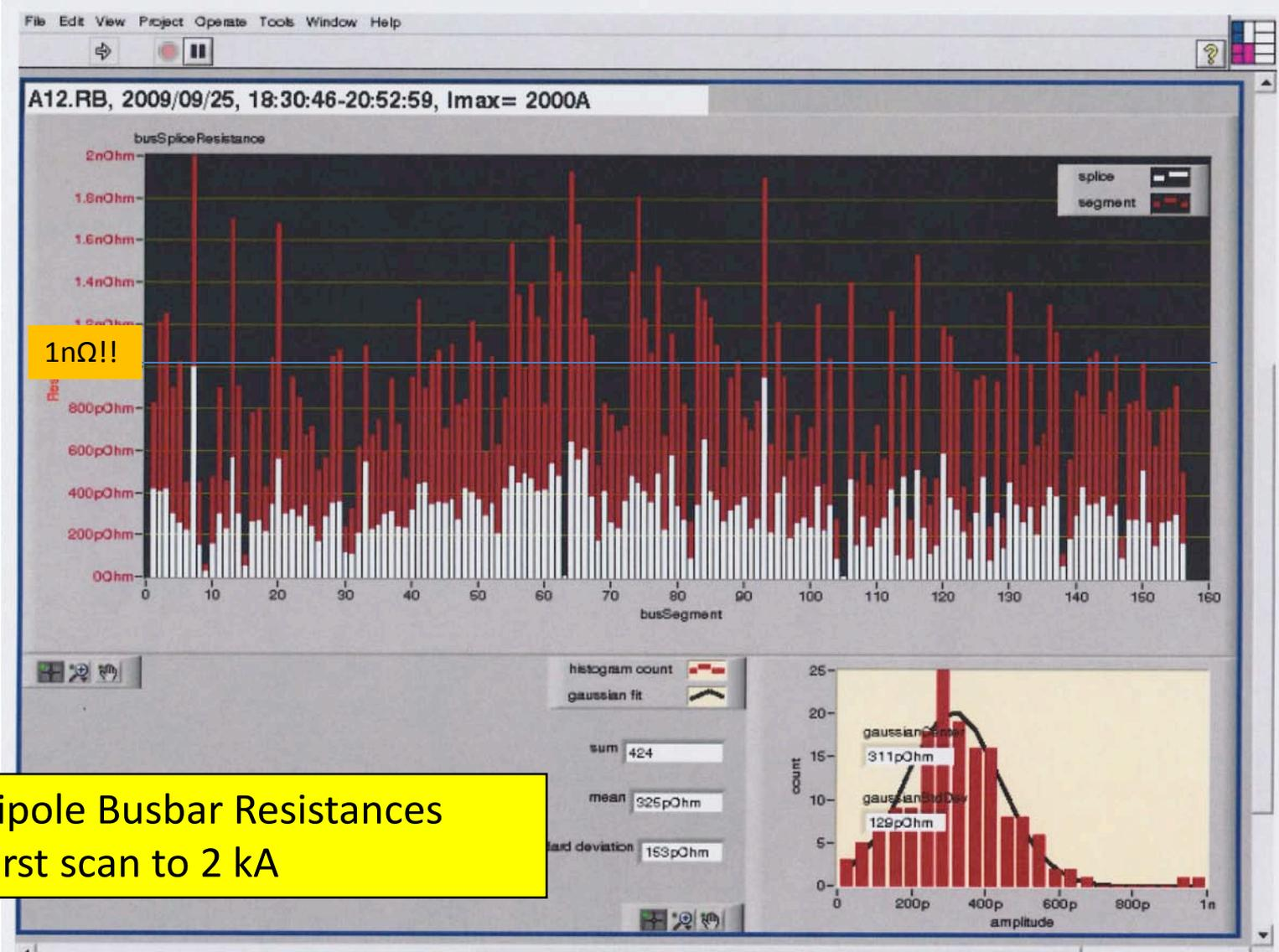
First Dipole Busbar Resistances from first scan to 2 kA
