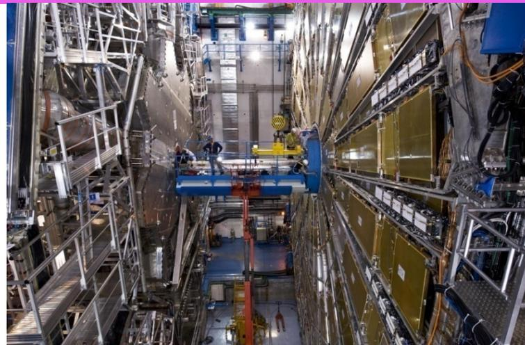
16<sup>th</sup> June closure of beam pipe & insertion of LUCID detector
