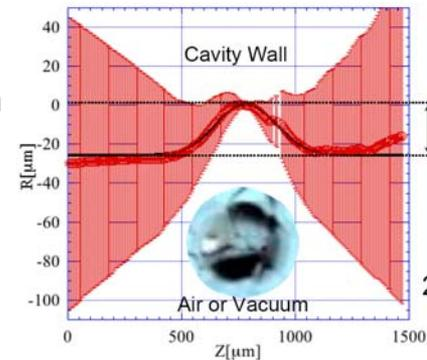
**Pit** found by KEK optical inspection with CCD camera in AES #1 cavity
