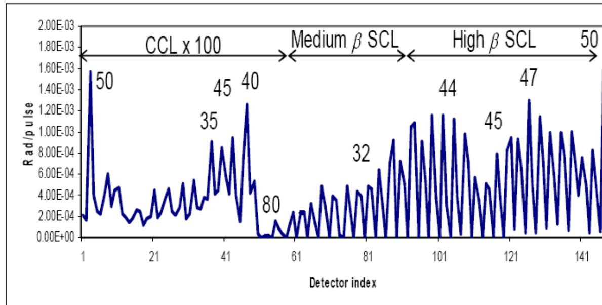
Figure 4: Linac beam loss monitor signals (rads/pulse) recorded during 475 kW operation. Numbers overlaid show residual dose rates (mrem/hr) at 30 cm measured ~24 hours after beam operation.
