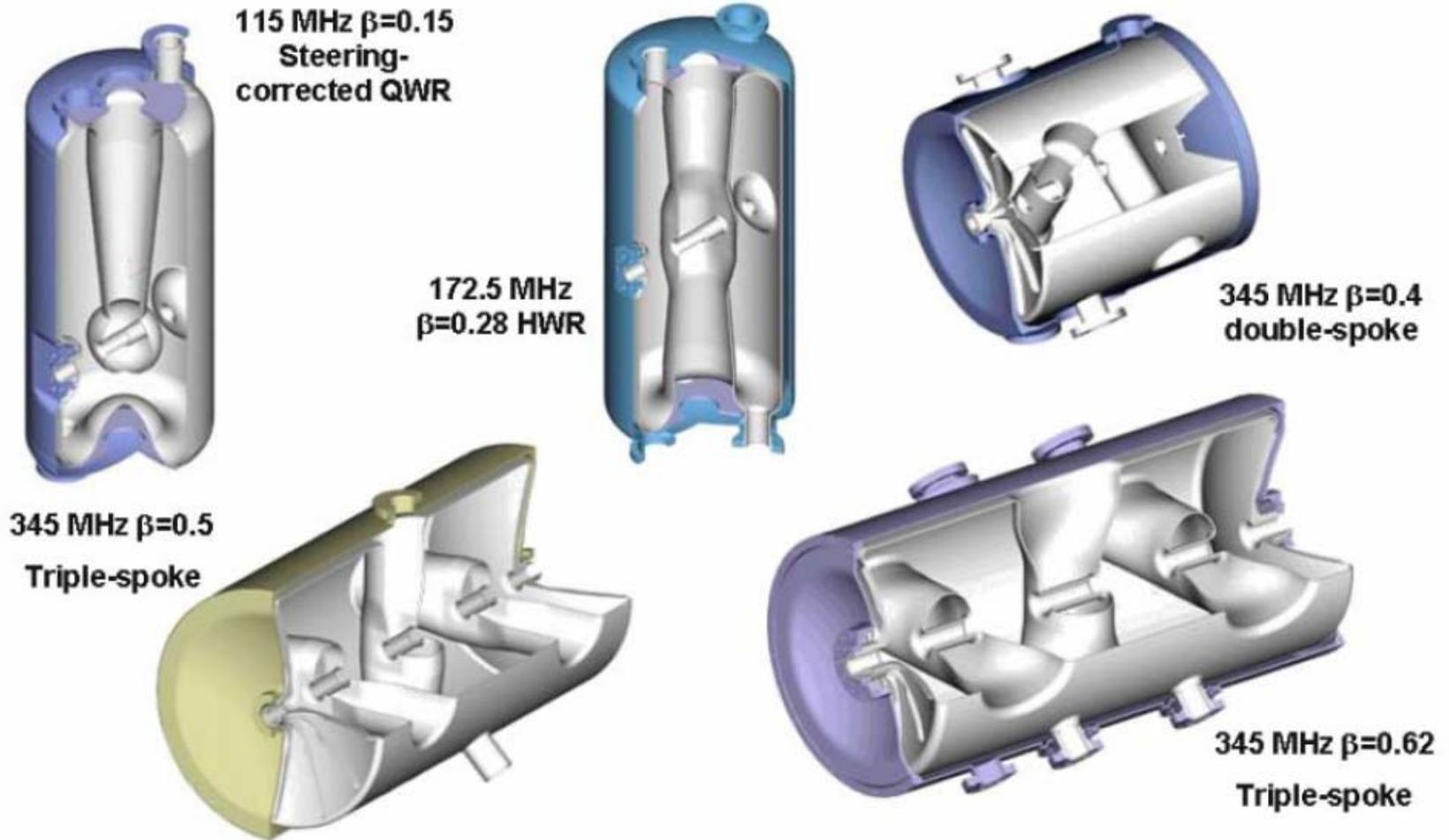
Figure 2: Five types of SC cavities developed for the AEBL driver linac.
