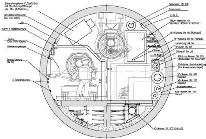
The ILC linear accelerator is proposed to be placed in the drift clay at the depth of 20 m with the idea that below the tunnel there should be impermeable soil preventing from the underlying groundwater intrusion. It is possible to construct tunnels of the accelerating complex using tunnel shields with a simultaneous wall timbering by tubing or falsework concreting.
