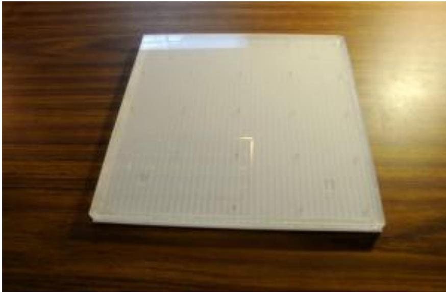
Complete assembly for 8" x 8" photodetector module .
