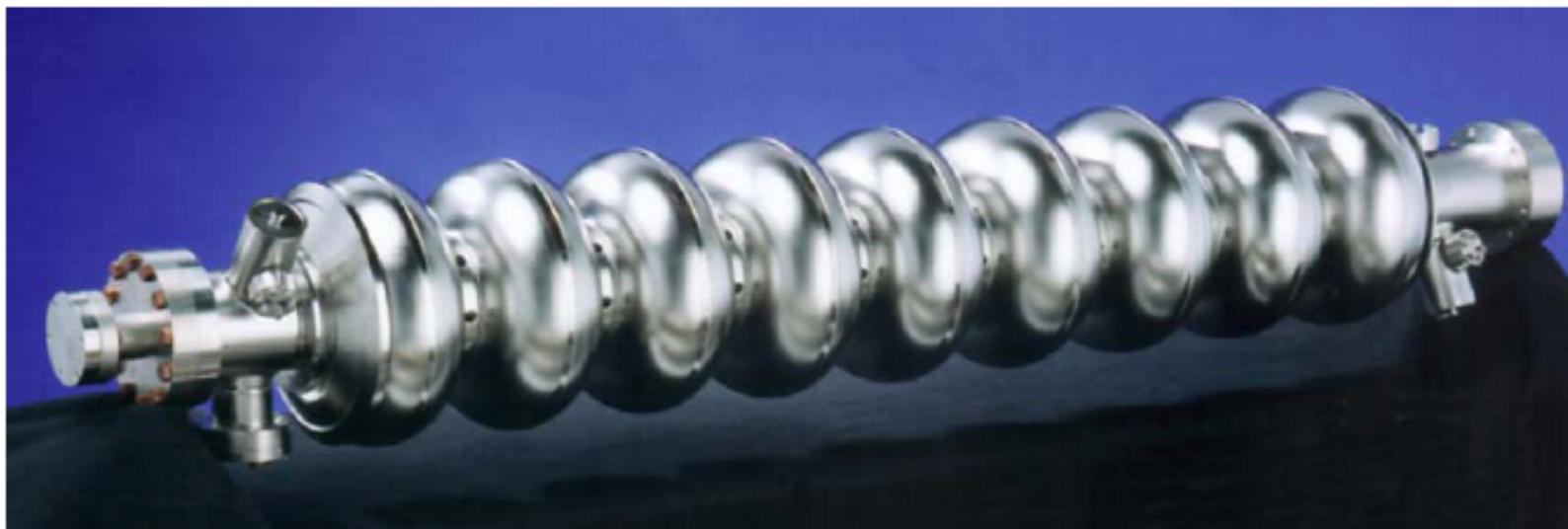
Figure 1.2-1: A TESLA nine-cell 1.3 GHz superconducting niobium cavity.
