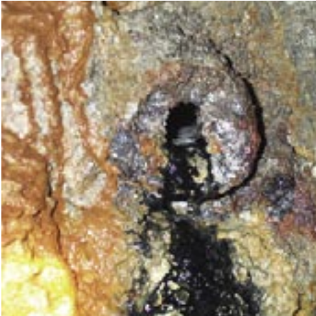
Biofilm: Black fluid emanating from a heavily corroded borehole at 3.1 km depth in the Mponeng gold mine in South Africa. The black fluid is due to “nanoparticles” of iron sulfide precipitated by thermophilic anaerobic sulfate-reducing bacteria and the corrosion is due to thermophilic aerobic sulfide and iron-oxidizing bacteria.
