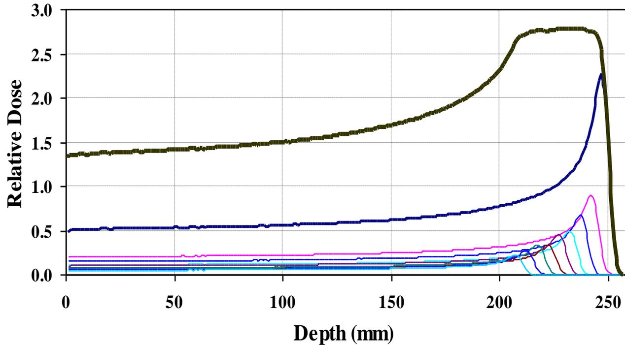
Adding together Bragg peaks from multiple beam energies with independent weights can generate a flat region at the tumor at the expense of increasing the entrance dose
